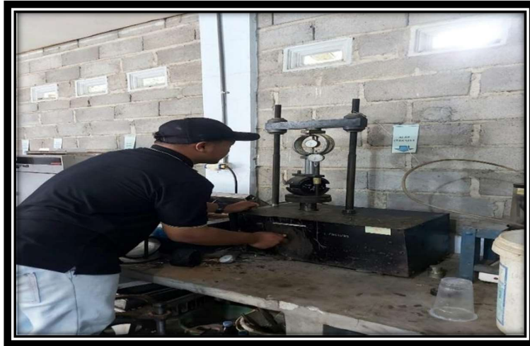
Gambar 22 : Pengetesan Benda Uji Marshall ( Test Stability)
