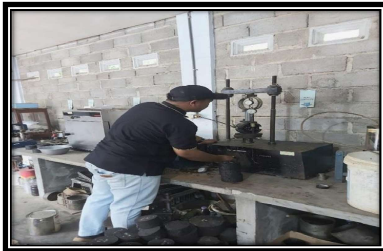
Gambar 23 : Pengetesan Benda Uji Marshall ( Test Stability)
