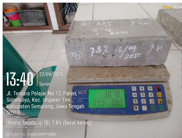
Gambar 3.5 Penimbangan Massa Kering Paving.
