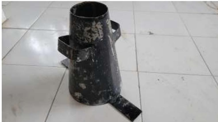
Gambar 3. 10 Kerucut Abrams
