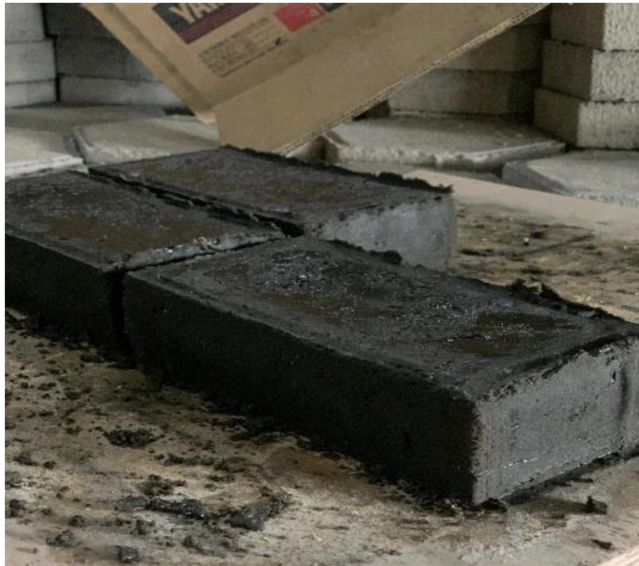
Gambar 3. 12 Proses Pengeringan Paving Block
