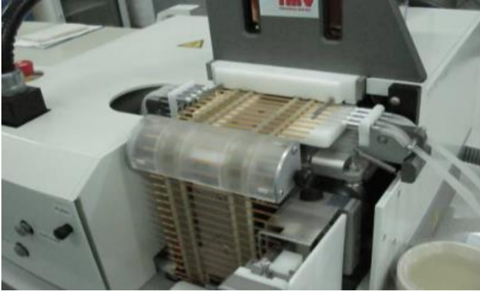
Gambar 20. Mesin filling and sealing (Sumber: Barszcz et al. ,2012)
