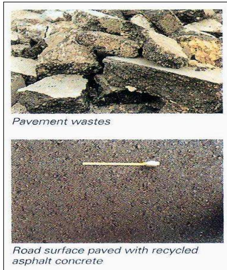
Figure 2.2. Pavement Wastes and Road Surface Paved with Recycled AC (National Construction Development Institution, 2013)
