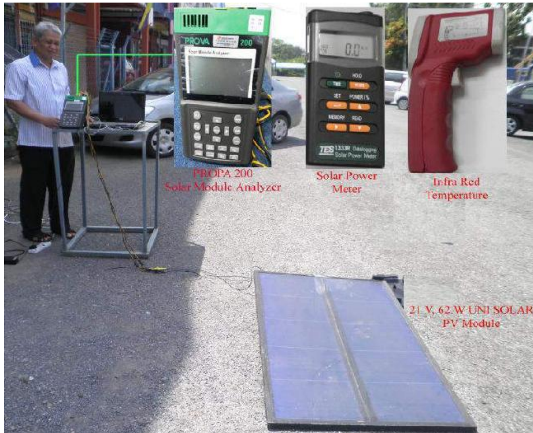
Figure 1 Measurement of PV module performance
