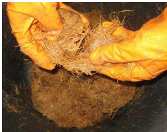
Figure 2 Mixing the EFB Fibers and Potato Binding Agent
